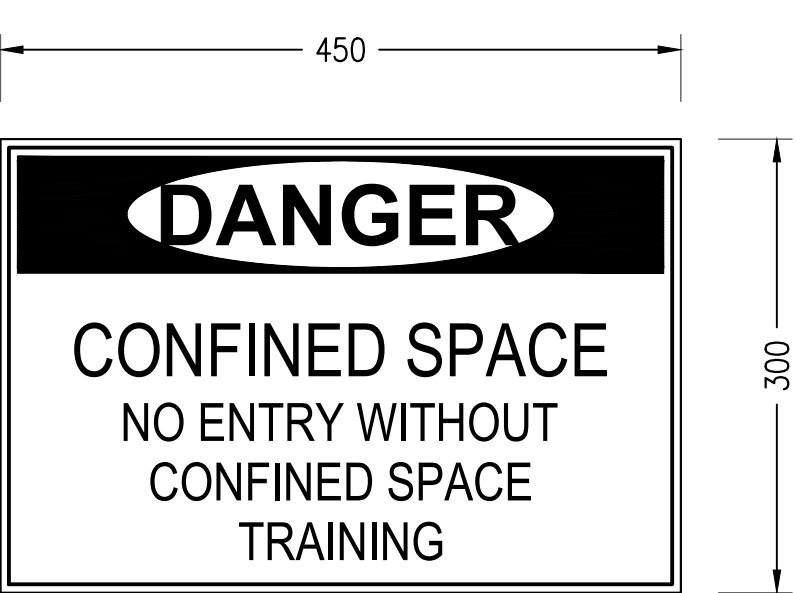
CONFINED SPACE SIGN DETAIL SCALE 1: 20
